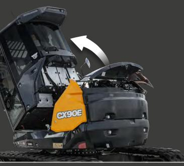
**TILTABLE CAB** With all maintenance points accessible from the ground.
